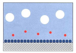
Polymerization occurs when the cyano, acrylic molecules change from a liquid substance to a hard structure. During polymerization, a chain of molecules is formed on the surface. Bonding is achieved by attracting the molecules of the material being glued. These links form a complex unit that creates bonding between two surfaces.
