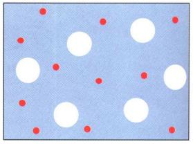
When the adhesive is applied to the surface, the stabilizer is neutralized by the alcanity of the substrate or by the residual moisture. Microscopic amounts of moisture are always present on surfaces that come into contact with the outside air.
